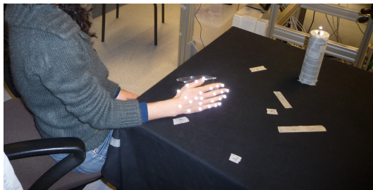
Figure 3.13: The markers on the object allow identifying its position.
